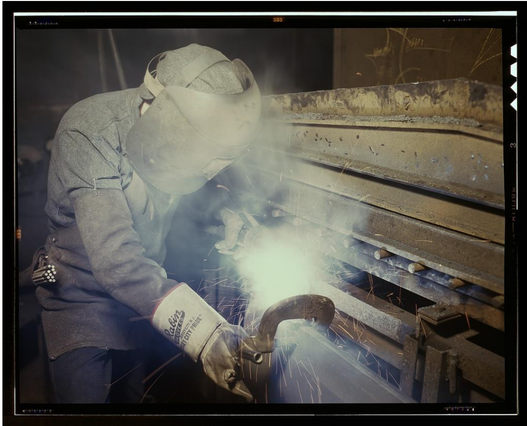
Alfred T. Palmer. Welder making boilers for a ship , Combustion Engineering Co., Chattanooga, Tenn. Tennessee, Estados Unidos / Estats Units. 1944. Library of Congress . Document sense restriccions conegudes de drets d'autor.
